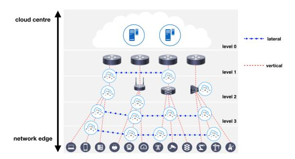
Figure 2.2.1: A typical fog architecture in a airport monitoring use case (source OpenFog [12]). The diagram demonstrates the need for lateral and vertical data sharing across different airport sub-systems and terminals at different fog levels.
