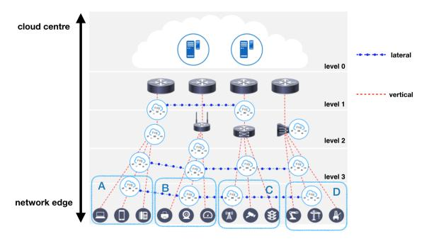
Figure 2.3.1: A typical fog architecture in a airport monitoring use case (source OpenFog [12]). The diagram shows the four Far edge regions where nodes are at a close proximity.
