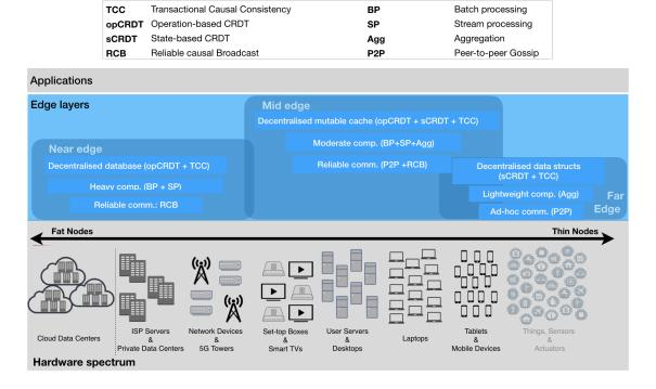
Figure 2.4.2: A figure that shows the characteristics of LiRA edge layers (in the three shaded tables). Within each edge layer, a type of decentralized lateral data sharing is used (Solution 1). Across the three layers, common semantics and possibly TCC are used to support convergent vertical data sharing (as specified in Solution 2). The used techniques shown in each layer are rough options that are likely to be used—although other options are possible.
