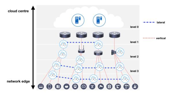
Figure 1.1.1: A typical hierarchical architecture for fog and edge computing in an airport monitoring use case (figure taken from [12]). The diagram shows both lateral and vertical data sharing across different airport sub-systems and terminals at different levels of the fog hierarchy.
